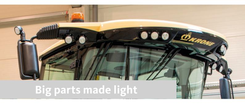
With know-how and the largest thermoforming machine of Europe we are able to substitute huge agricultural machine parts with light plastic. We deliver completely mounted bonnets, roofs and much more directly to your production line.
